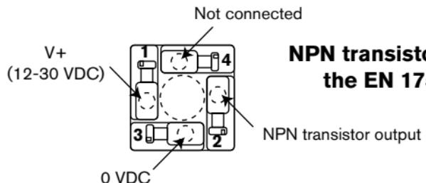
**NPN transistor output connection of
