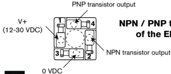
**NPN / PNP transistor output connection
