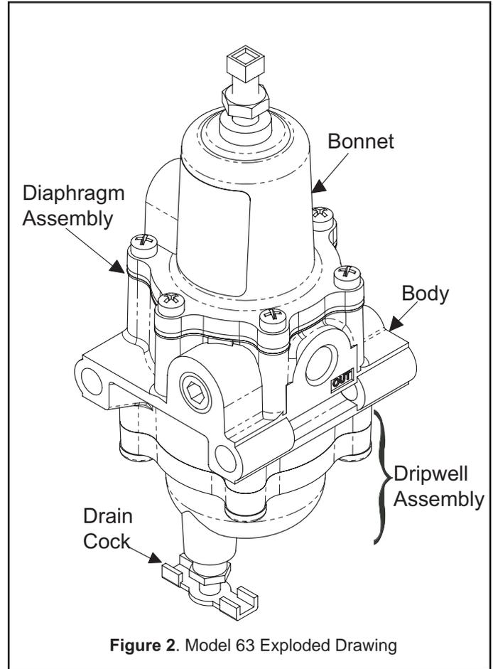
**Figure 2.** Model 63 Exploded Drawing
