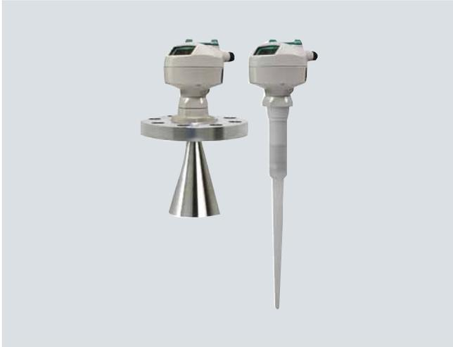
SITRANS LR200 is a 2-wire, 6 GHz pulse radar level transmitter for continuous monitoring of liquids and slurries in storage and process vessels including high temperature and pressure, to a range of 20 m (66 ft).
