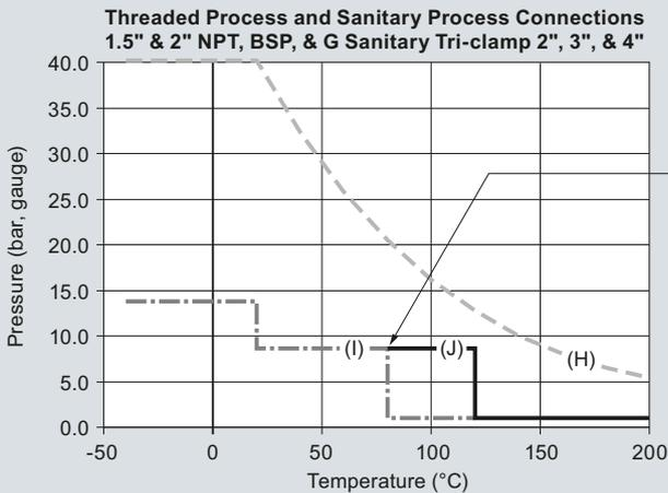
UHMW-PE is limited to 80 °C, it can be used to 120 °C for short (3 hrs) durations at ambient pressure, no stress applied to the antenna.
