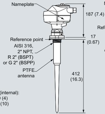
**Threaded Connection PTFE Rod, external shield**
