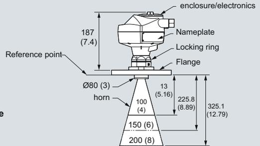
**Waveguide Antenna with Flat Faced Flange**
